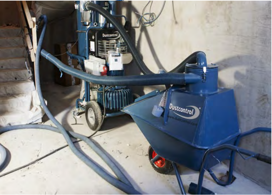
DC 5900, 9.2 kW P central unit with DC F Wheelbarrow pre-separator.
